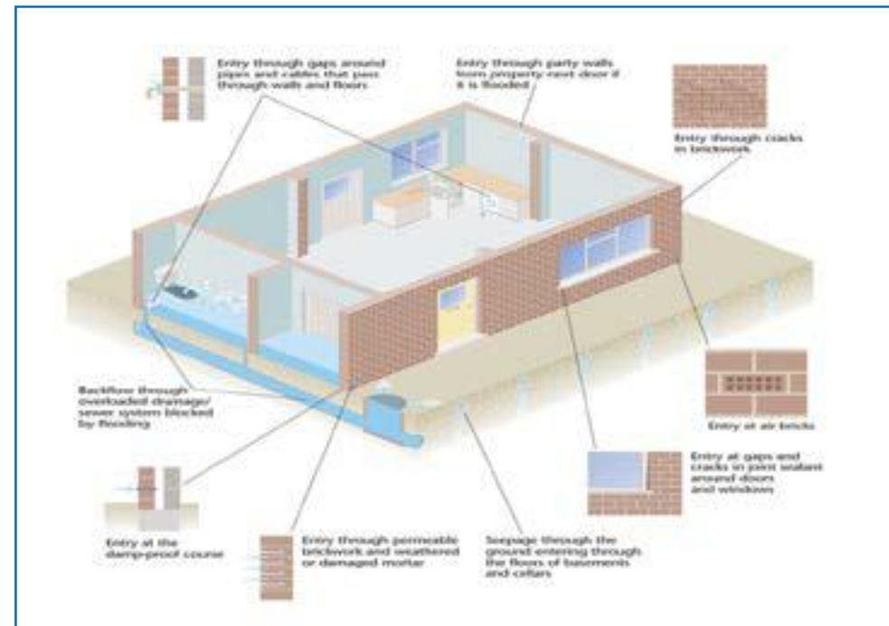
Doors, low windows, air bricks, broken brickwork, backflow up through the toilet, ground water 'rising up' under the floor, are just a few of the many ways water can enter a property.
